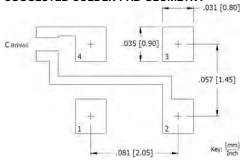
$C_{BYPASS}$  should be  $\geq 0.01$  uF.
