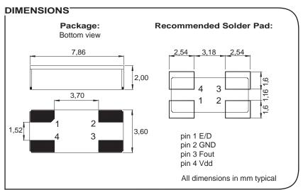
**SMT Clock oscillator in ceramic** package Fundamental quartz mode frequency High shock and vibration resistance Wide temperature range Low aging **Ultra low MSL** Very fast start-up **Excellent solderability** Swiss made quality **Customer specification on request**
