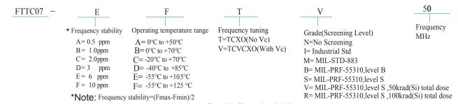
Freq. Vs Temp Availability C: ±2.0ppm Temp (°C) A: ±0.5ppm B: ±1.0ppm D: ±3.0ppm E: ±6.0ppm A: 0°C to +50°C B: 0°C to +70°C ٠ C: -20°C to +70°C 0 D: -40°C to +85°C 0 -55°C to +105°C 0 0 0 -55°C to +125°C 0
