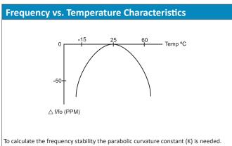
For calculating the stability at 45°C? 1- Change in temperature ( $\Delta$ T) is (45-25) = +20°C 2- Change in frequency is (-0.034 x ( $\Delta$ °C)²) = (-0.035 x (20)² = -13.6ppm
